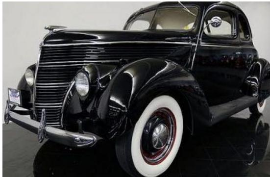
Whitewalls have a very simple origin story: pure rubber doesn't wear all that well, and one of the early success stories in mixing chemical compounds into tires to add longevity was zinc oxide. This had the side effect of creating a completely white tire, and by the time carbon black arrived on the scene to
