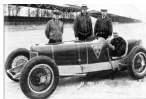
Rookie Indy 500 driver Al Miller was about to try out the Buddy Marr- owned Hudson Special before the 1932 Indianapolis 500. It featured a lot of stock parts including a 254 cid straight eight.
