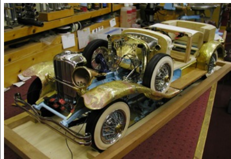
The bodywork is all metal, not fibreglass. Here is the car in Lou's shop before the brass coachwork was primed or painted. Lou is not adverse to remaking a part that doesn't meet his standards. He started over on the especially difficult brass radiator shell nine times.
